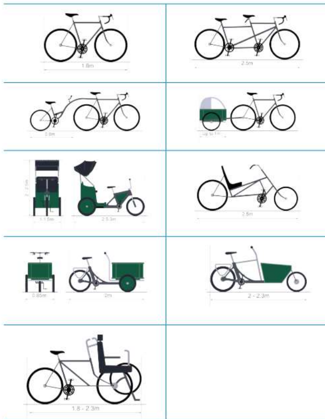
Figure 5.2: Typical dimensions of cycles
